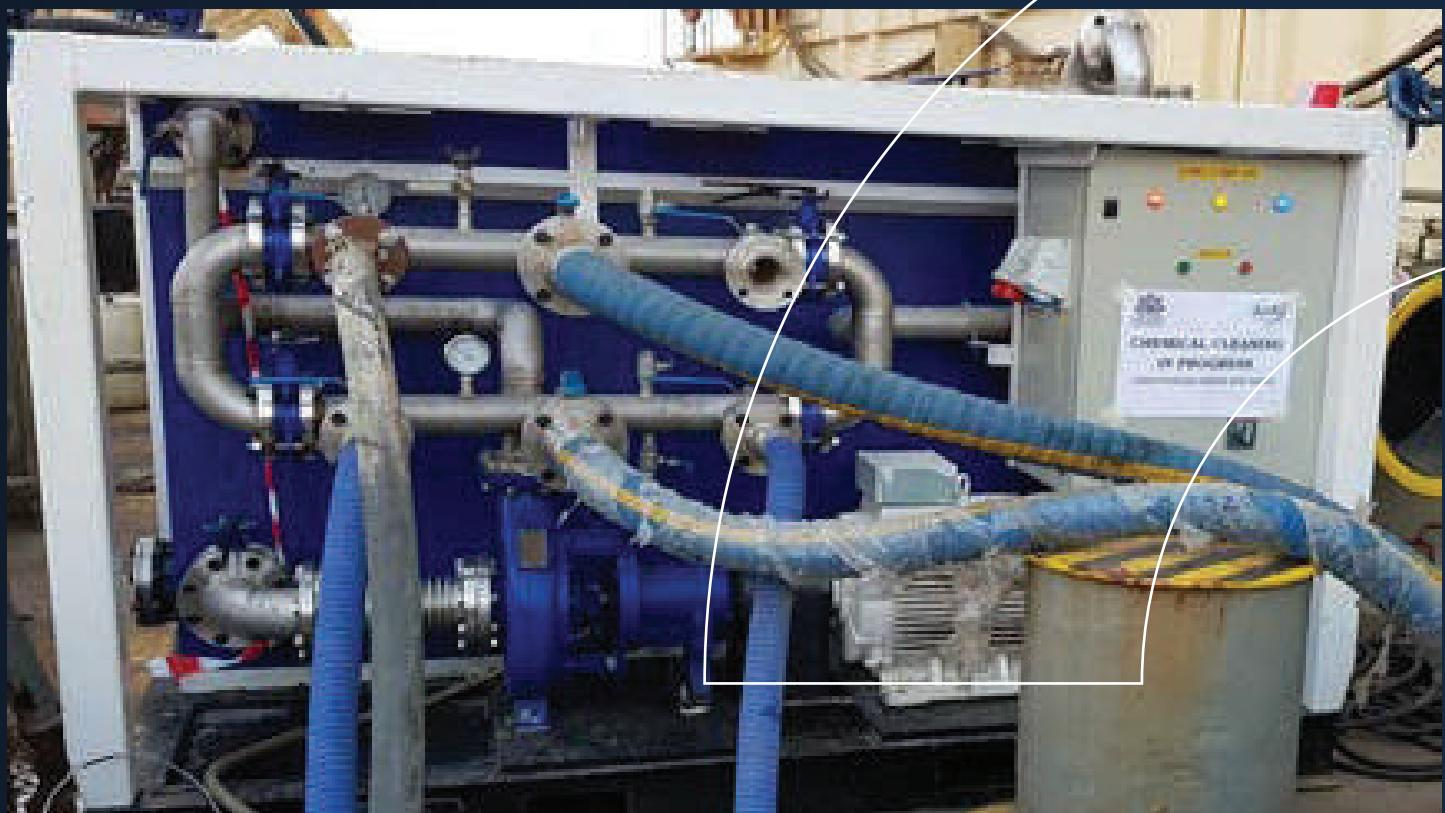
**AM Boiler** is dealing with chemical cleaning of various metallurgies such as; carbon steel, stainless steel, cupro nickel, aluminum brass, titanium etc. Our highly skilled chemical engineers carry out a thorough analysis to identify the optimum cleaning method ensuring it will successfully remove the fouling without negatively affecting the process equipment.
